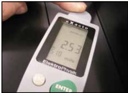
Coating Thickness Test Coating thickness is measured and plotted every hour.
