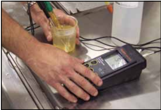
System Titration Test Ph levels are checked twice per shift as part of the pretreatment titration check.
